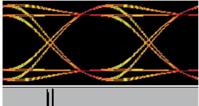
Figure 4.2.4c. An Eye Diagram and Histogram of Data Dependent Jitter.
