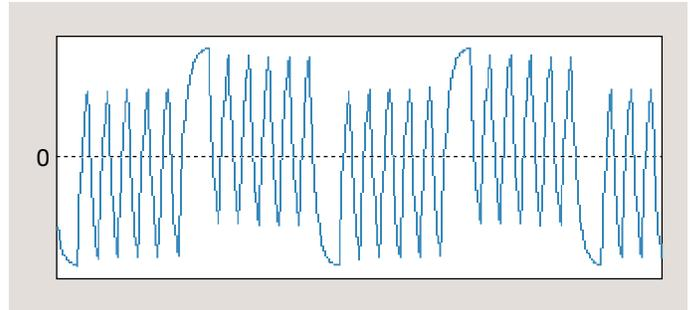
Figure 4.2.4a. Data Signal with Data Dependent Jitter.
