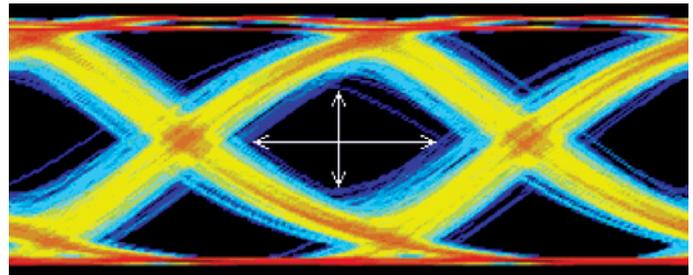
Figure 3.5b. A Waveform Database with Color Gradation.
