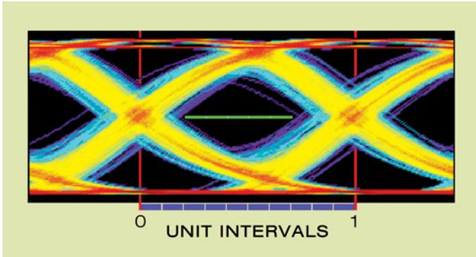
Figure 5.2a. Eye Width is used to Determine Performance.
